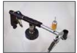
Screw in the new teflon tube
