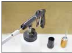
Slide the box spanner over the teflon tube and tighten it.
