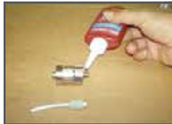
Apply some Loctite before mounting the new aluminium tube.
